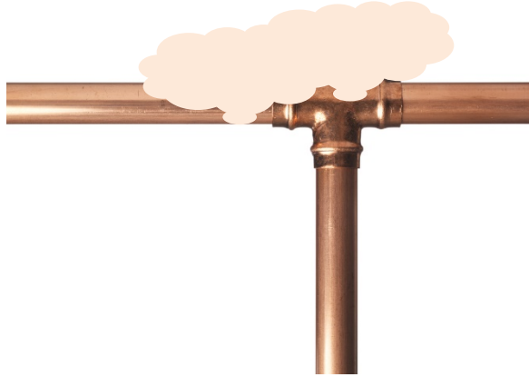
Fig 4.10.15: Leak detection using soap solution
