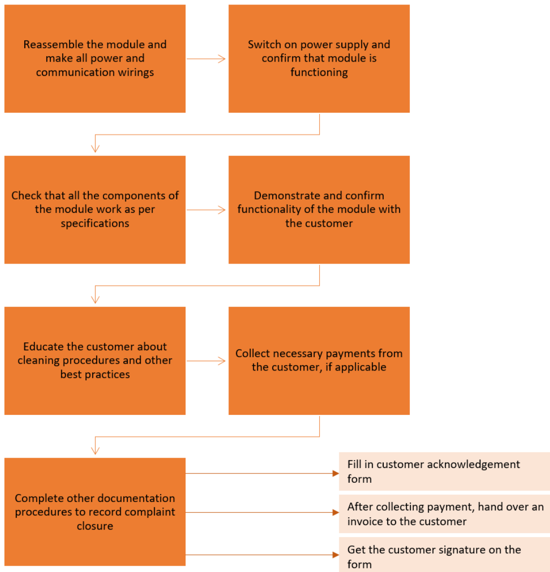
Fig 4.9.4: Steps to confirm functionality of the repaired unit
