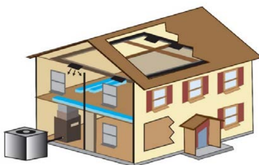
Fig. 1.3.6: A central AC system
