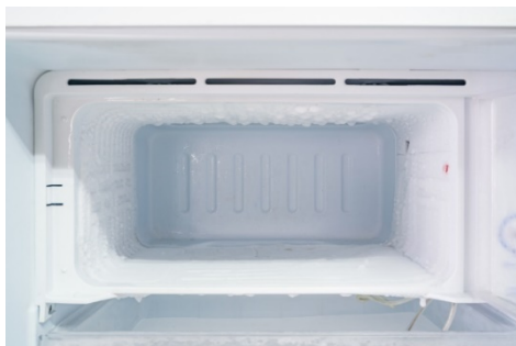
Fig 4.6.5: Frost formation in the freezer of DC refrigerator
