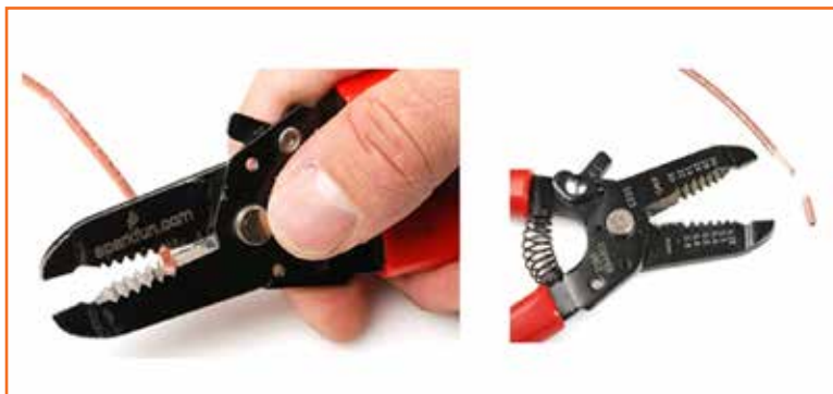
Fig 2.4.3 Stripping of wire
