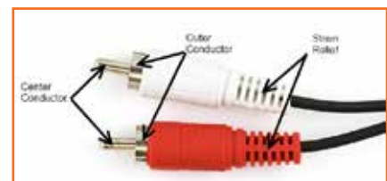
Fig 2.2.75 RCA Connector
