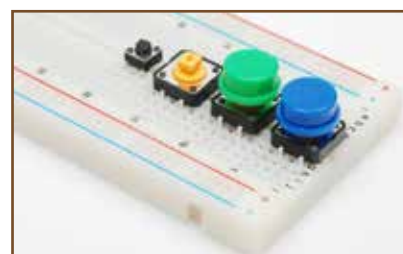
Fig 2.2.3 Mounting style switches
