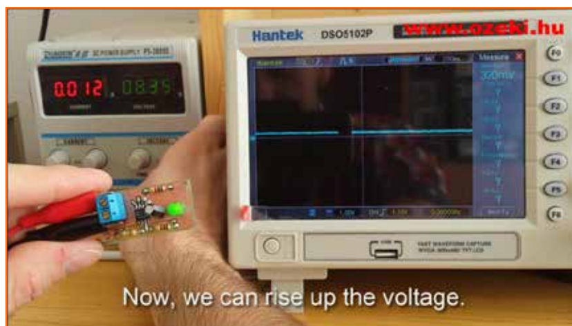
Fig 3.1.12: Checking PCB by oscilloscope
