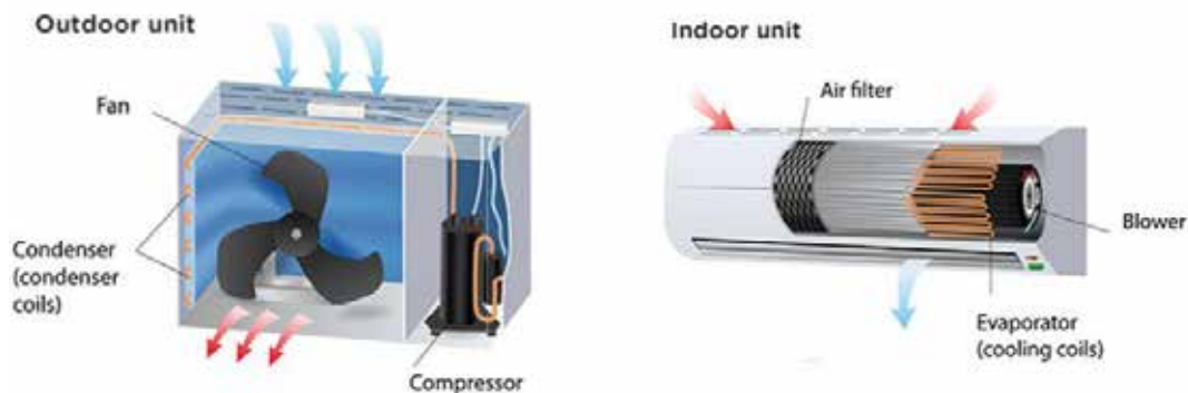
Fig. 1.2.18: Split System HVAC
