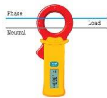
Fig. 4.3.6: Testing a single-phase circuit
