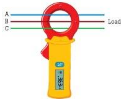
Fig. 4.3.7: Testing a three-phase circuit
