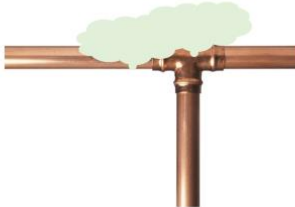
Fig. 4.2.14: Leak detection using soap solution
