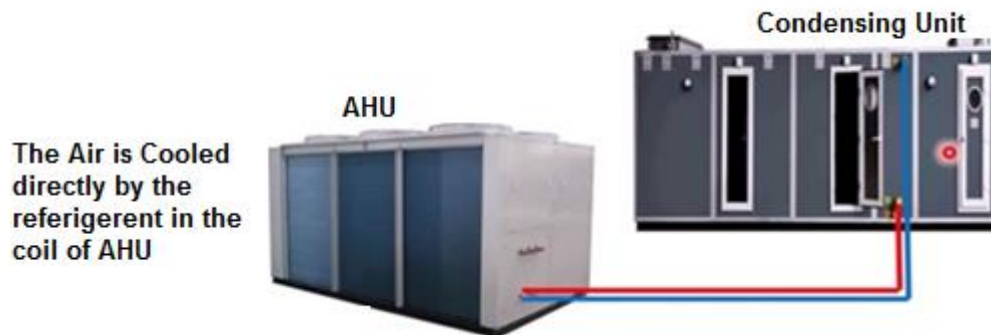
Fig. 1.2.22(a): Direct Expansion Fresh Air Handling unit (DX FAHU)
