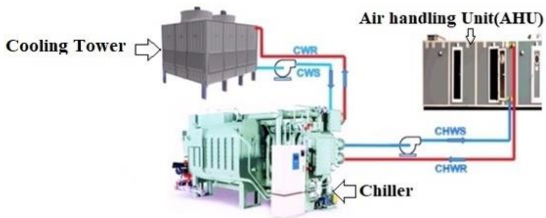
Fig. 1.2.25: Chilled Water Air Conditioning System
