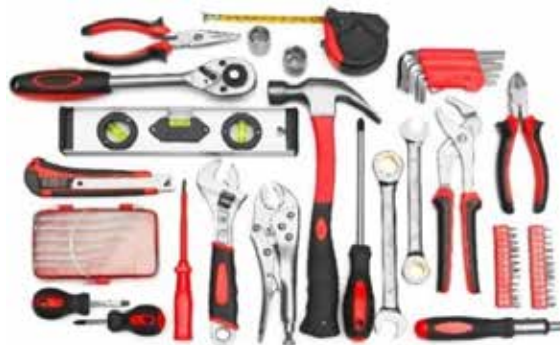
Fig. 1.4.1: Hand tools used in RAC components' assembling
