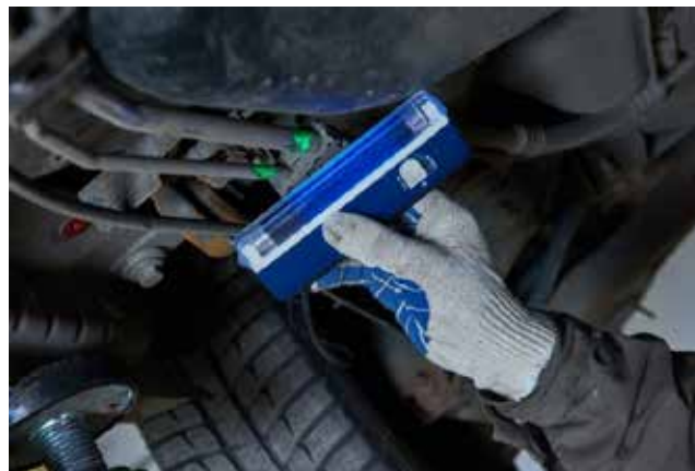
Fig. 4.2.15: Leak detection using ultra-violet lamp
