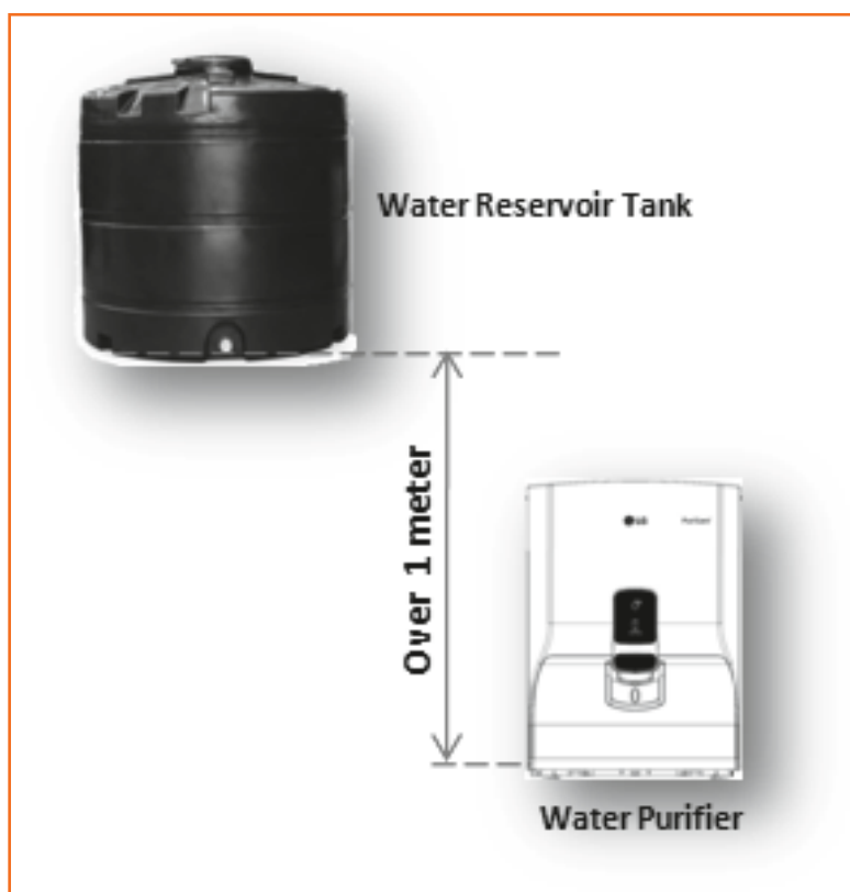
Fig 5.5.3 Installation of water purifier
