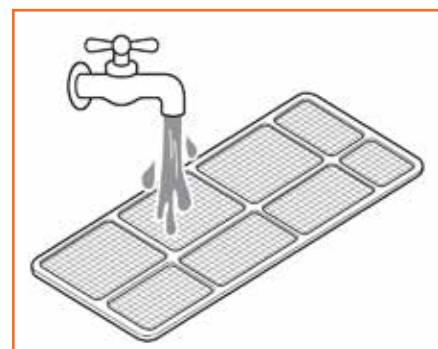
Fig 5.2.20 Cleaning of air filter
