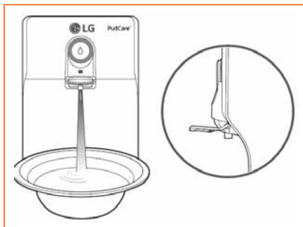
Fig 5.6.2 Draining water from water purifier
