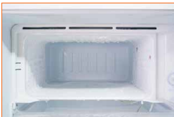
Fig 2.1.15 Frost formation in the freezer of DC refrigerator
