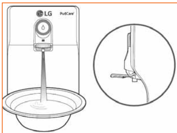
Fig 5.6.8 Draining water from water purifier
