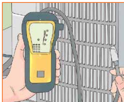
Fig 6.2.6 Electronic leak test
