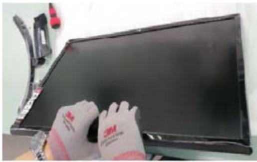
1. Disassemble from top -> left/right -> top corner .
