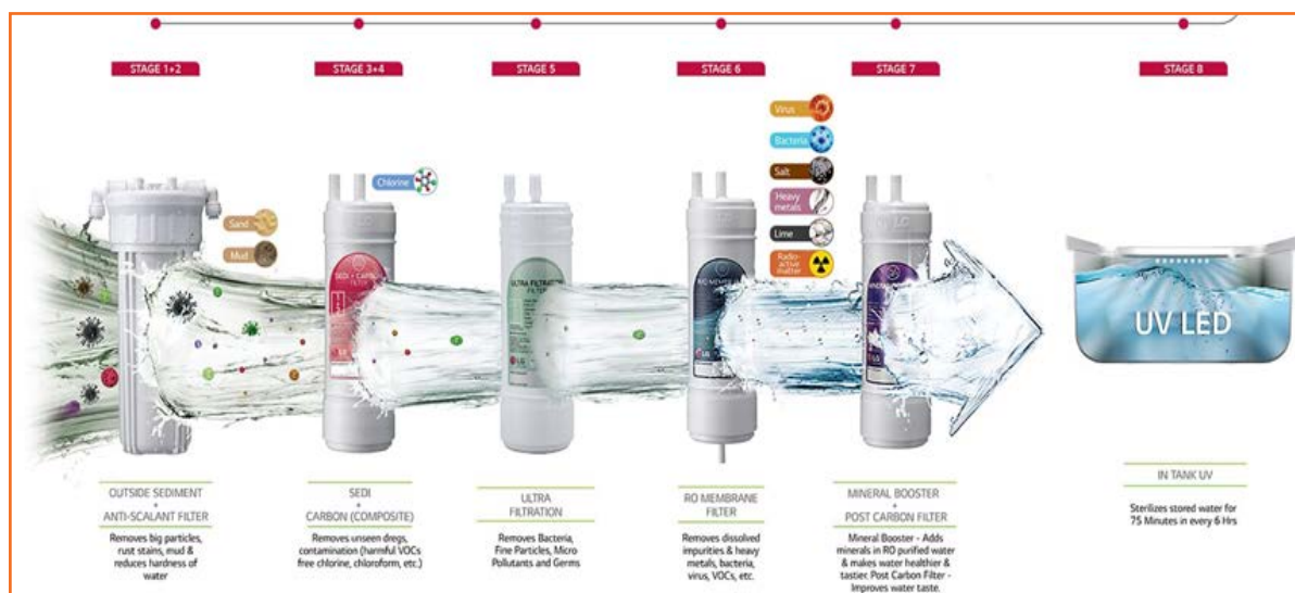
Fig 4.1.10 Multi stage filtration process
