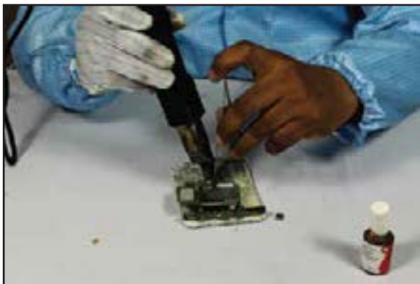
Fig: 3.3.7.1.4 Charging Connector Soldering - Step 1
