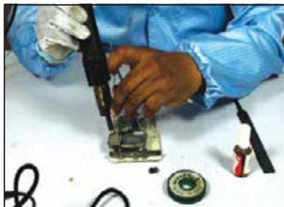
Fig: 3.3.7.3.3 Headphone Connector Soldering - Step 2
