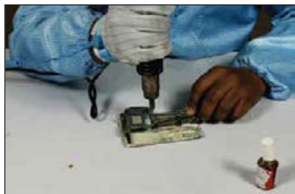
Fig: 3.3.7.1.2 Soldering Flux on Charging Connector
