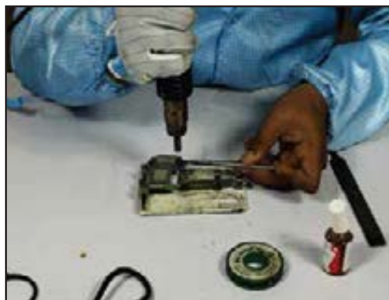
Fig: 3.3.7.3.2 Headphone Connector Soldering - Step 1
