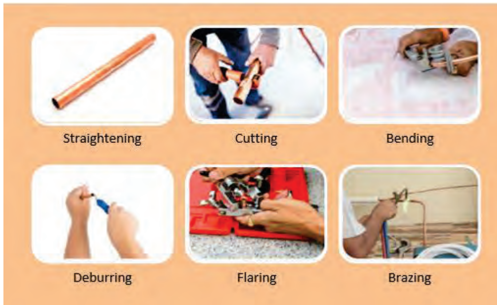
Fig 6.1.1: Copper tubing operations in RAC
